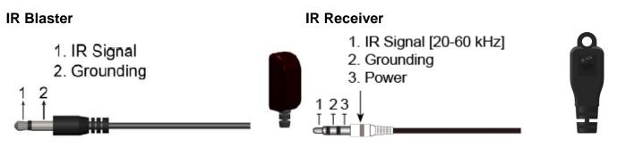
You can buy any IR extension cables in the market that are compatible to the definition of the IR sockets for the matrix if necessary for replacement use. However, IR cables longer than 2m (6-ft) may not work.
